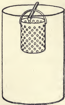
FIG. 24.—Precipitating vessel with contrivance showing how the zinc shavings are suspended.
