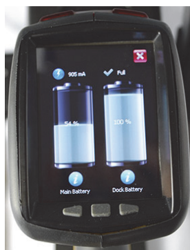
Figure 4-2 Battery charge status
