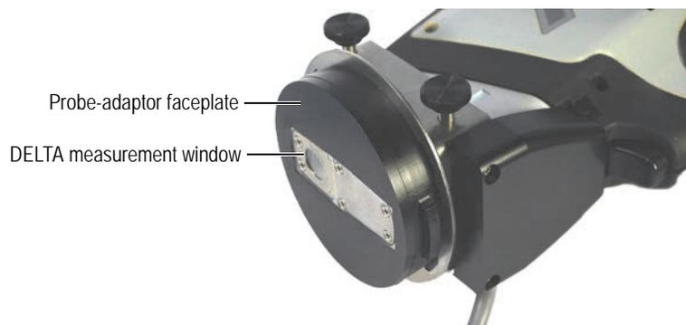
**Figure G-11 The DELTA measurement window flush with the probe-adaptor faceplate**
