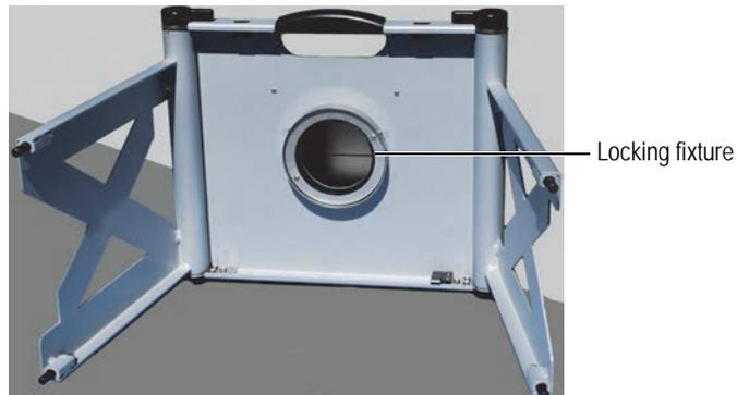
**Figure G-12 The test-stand locking fixture**
