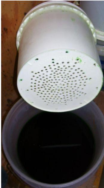
I typically agitate the bath twice a day by pulling the strainer out, waiting a moment or two, then slowly letting it back down into the bath. This causes the gold foils to go into the solution thru the bottom of the strainer and separates them from the finger boards.
